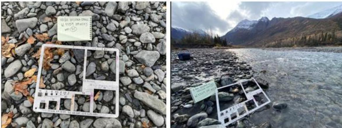
**Figure 1-4** Typical substrate observed in the lower 3.0 miles of East and West forks of Eklutna Creek. A gravelometer was used to categorize substrate size.
