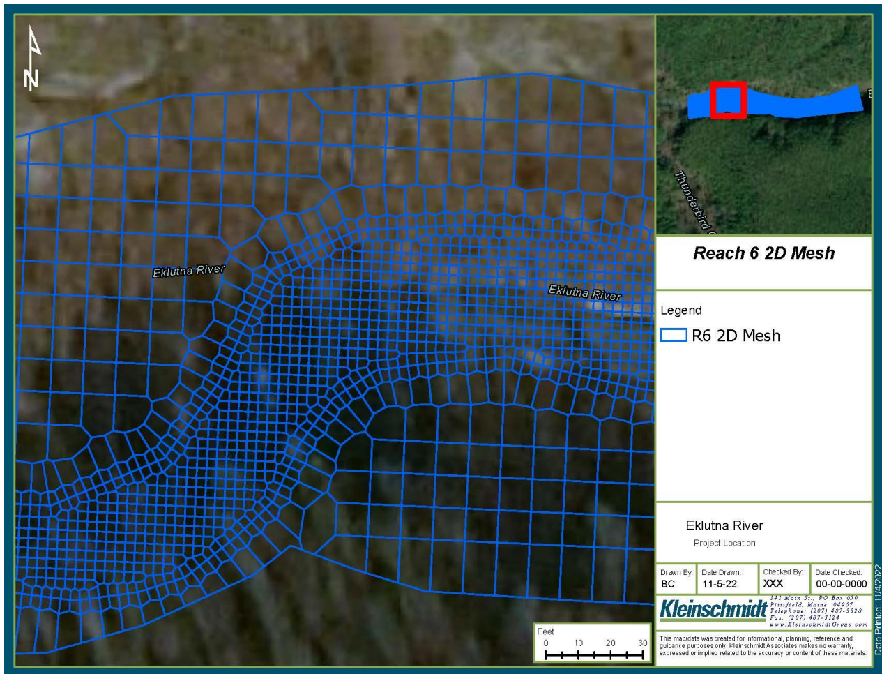
Figure 4-3 Subsection of Reach 6 of the Eklutna River illustrating the mesh cell sizes used in main channel and floodplain habitats. Smaller mesh sizes were used in the main channel to define complex habitat features. This segment of R6 was 1,167 ft long and contained limited side channel and off-channel habitats.
