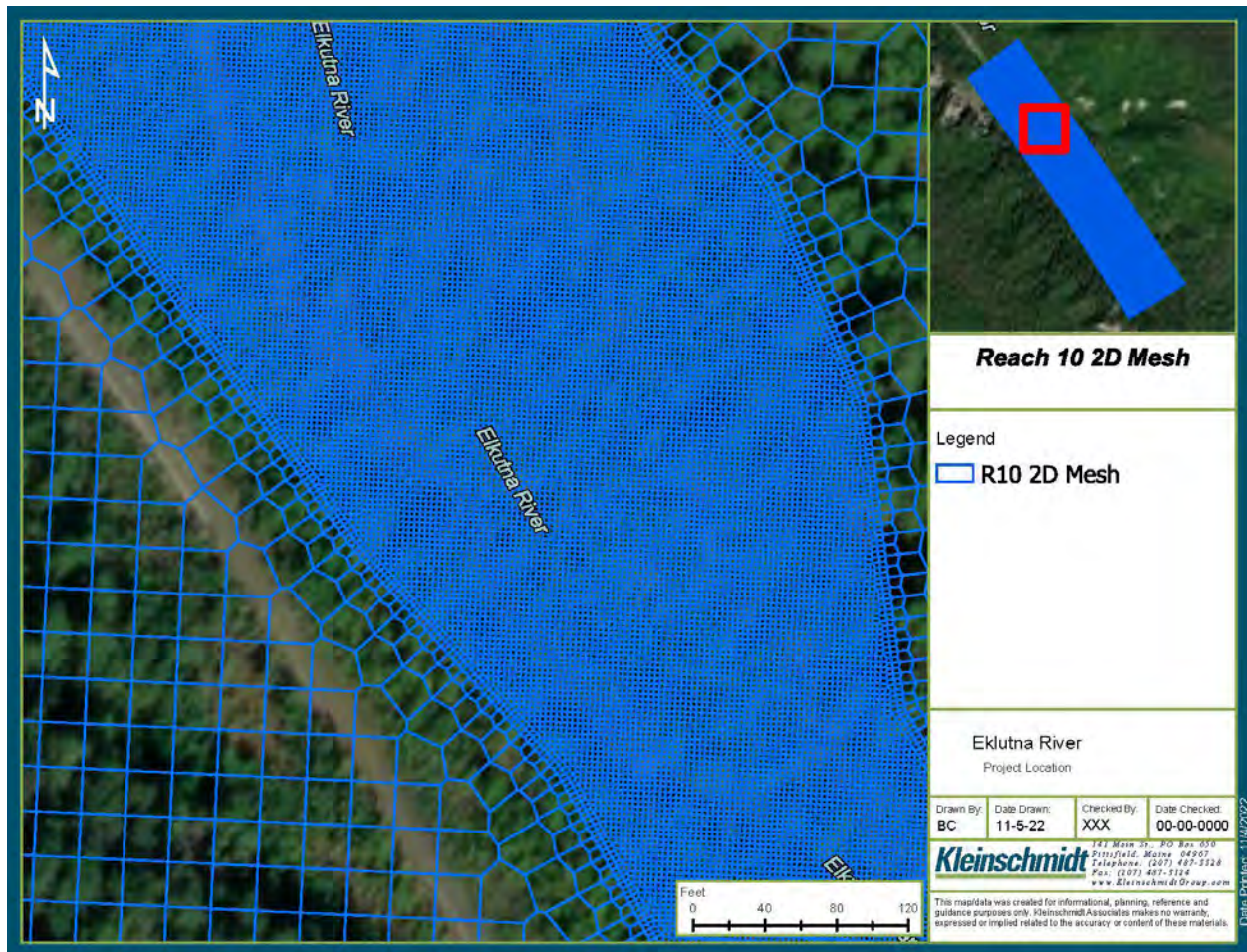
Figure 4.4-1. Subsection of Reach 10 of the Eklutna River illustrating the mesh cell sizes used in main channel and floodplain habitats. Smaller mesh sizes were used in the main channel to define complex habitat features. This segment of R10 was 3,744 ft long and contains representative side channel and off-channel habitats.
