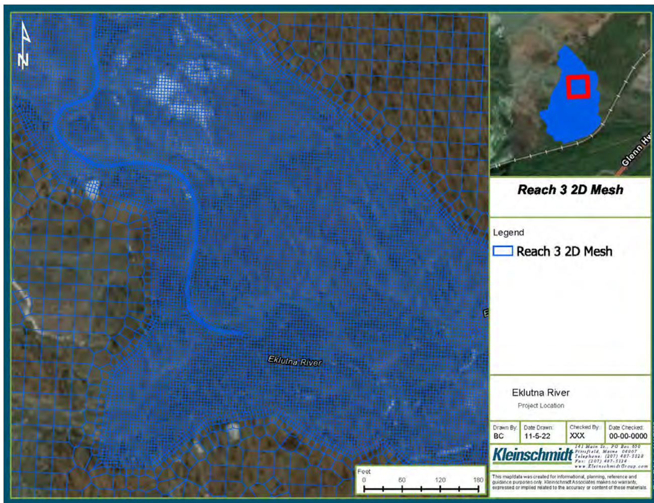
Figure 4.4-4. Subsection of Reach 3 of the Eklutna River illustrating the mesh cell sizes used in main channel and floodplain habitats. Smaller mesh sizes were used in the main channel to define complex habitat features. This segment of R3 was 2,183 ft long and contains a braided beaver complex and other representative side channel and off-channel habitats.
