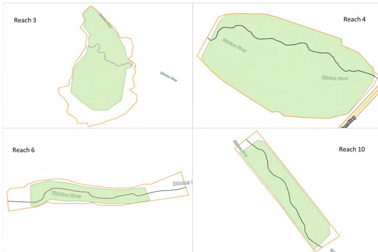
Figure 4.1-2. Model extents for each of the four reaches. The polygon border in orange represents the extent of the hydraulic model and the polygon in light green is the habitat model extent. Nominally, the models for Reaches 3, 4, 6, and 10 were 2,183 ft., 2,502 ft., 1,167 ft, and 3,744 ft in length, respectively. The line passing the middle of each polygon represents the main water course at low flow.
