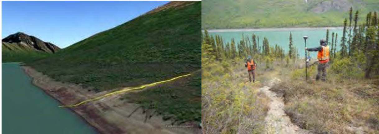
Figure 3.1-4. Visualized RTK data (left) of stream surface elevation for West Bank Tributary B and photograph (right) of tributary aspect and gradient. Data collected June 3, 2021.
