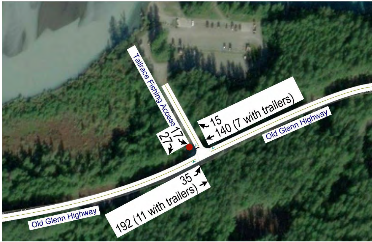
Figure 5: Vehicles on Old Glenn Highway and Turning into and out of Tailrace Access (6/11/2022 from 2 to 4 PM)
