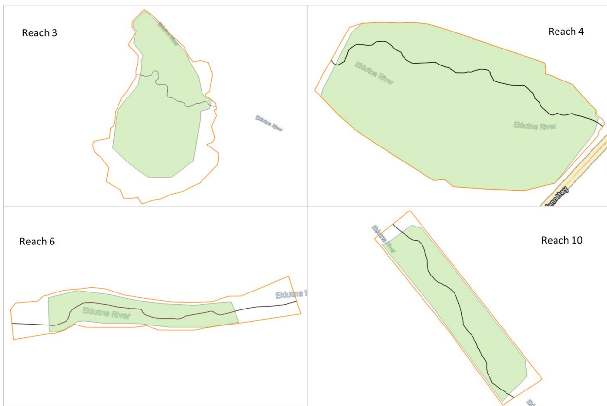
Figure 2-1 Model extents for each of the four reaches. The polygon border in orange represents the extent of the hydraulic model and the polygon in light green is the habitat model extent. Nominally, the models for Reaches 3, 4, 6, and 10 were 2,183 ft., 2,502 ft., 1,167 ft, and 3,744 ft in length, respectively. The line passing the middle of each polygon represents the main water course at low flow.
