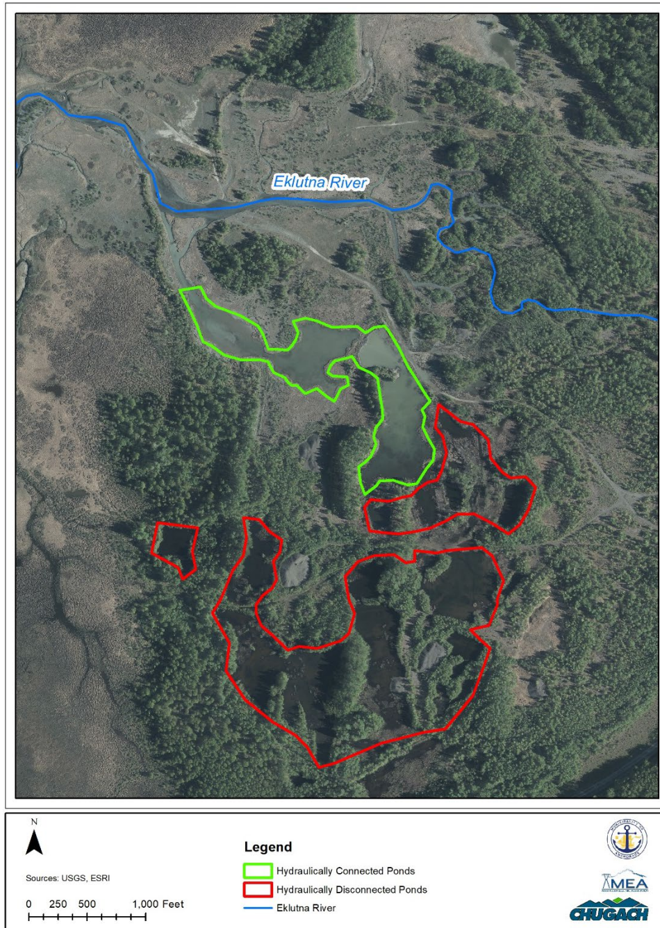
Figure 3-4 Off Channel Ponds located in Reach 3 of the Eklutna River. Some of these ponds may become physically connected to the river via surface flows, while others may remain disconnected with water levels influenced by groundwater from other sources or hyporheic underflow from the river.
