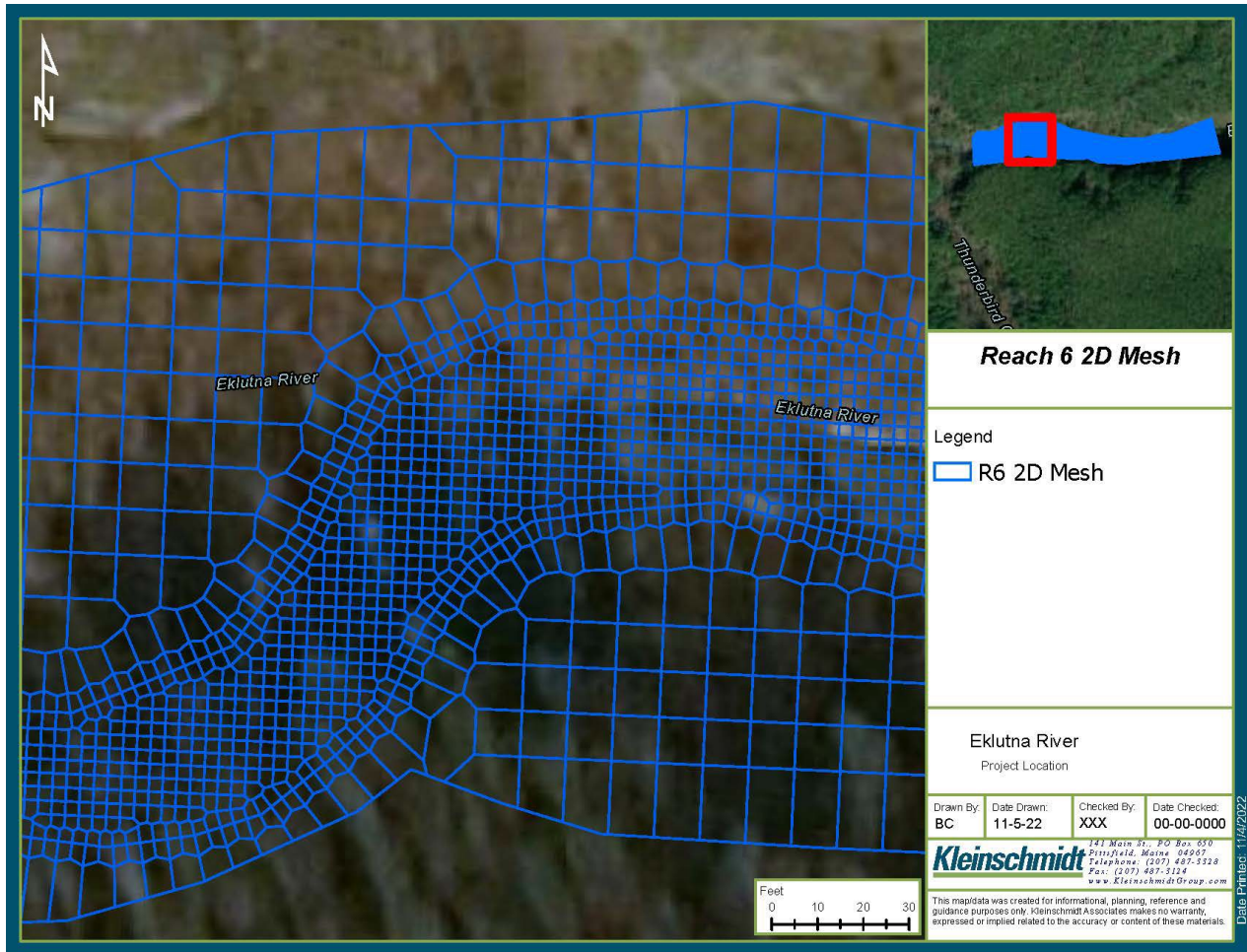
Figure 4.4-2. Subsection of Reach 6 of the Eklutna River illustrating the mesh cell sizes used in main channel and floodplain habitats. Smaller mesh sizes were used in the main channel to define complex habitat features. This segment of R6 was 1,167 ft long and contained limited side channel and off-channel habitats.
