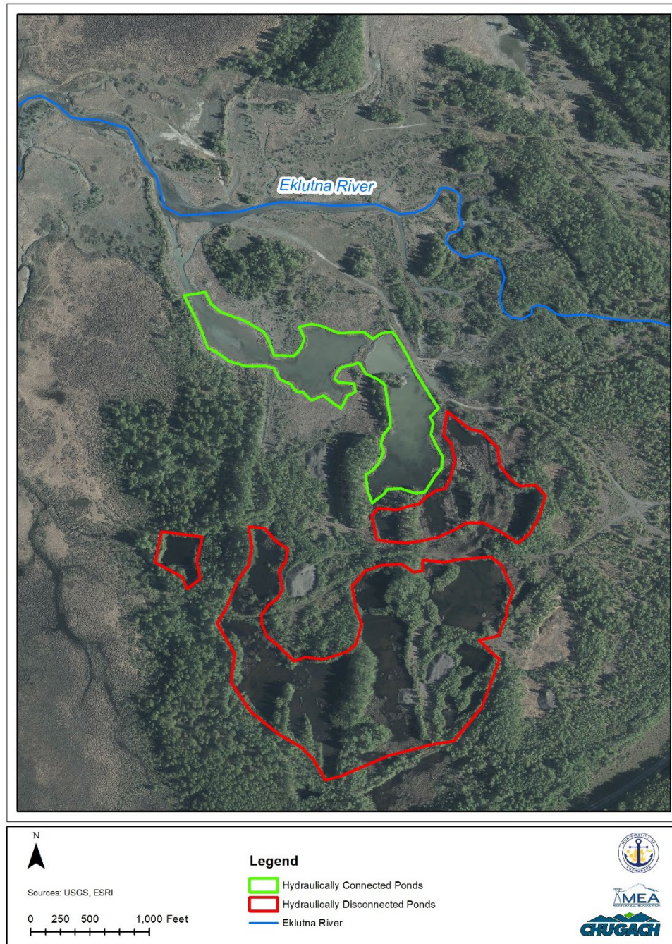
Figure 4.3-2. Off Channel Ponds located in Reach 3 of the Eklutna River. Some of these ponds may become physically connected to the river via surface flows, while others may remain disconnected with water levels influenced by groundwater from other sources or hyporheic underflow from the river.
